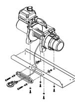
make sure the motor, drum and gearbox housing are aligned correctly.
