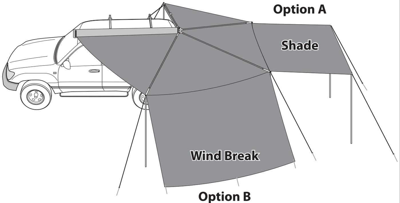
**Note :** The poles and ropes must always be used when the FOXWING awning is open
