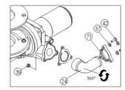
2. Impeller may get stocked inside pump body if the electric pump is idled for a period of time. Follow the indicated direction to rotate the impeller from outside to prevent the electric pump from damage of instant high current in starting operation.
